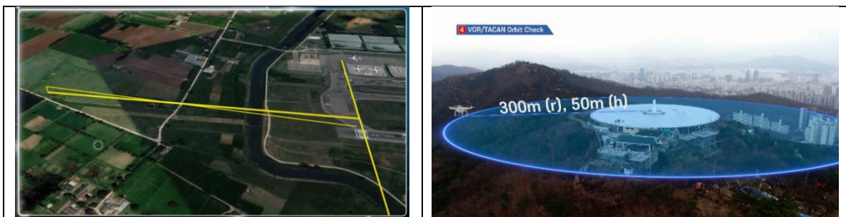
Figure 4. Drone automatic flight path for ILS and VOR check
