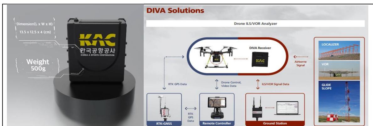
Figure 2. Drone system configuration diagram for navigational Aids check and software for analysis
